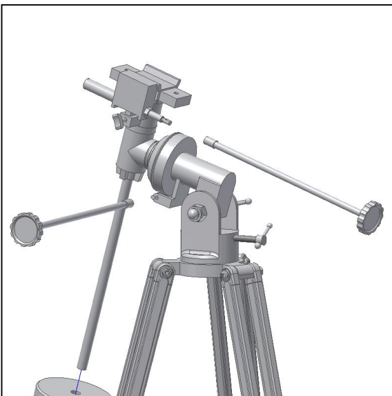
Figure 6. Fix Dec. and R.A. handles.
