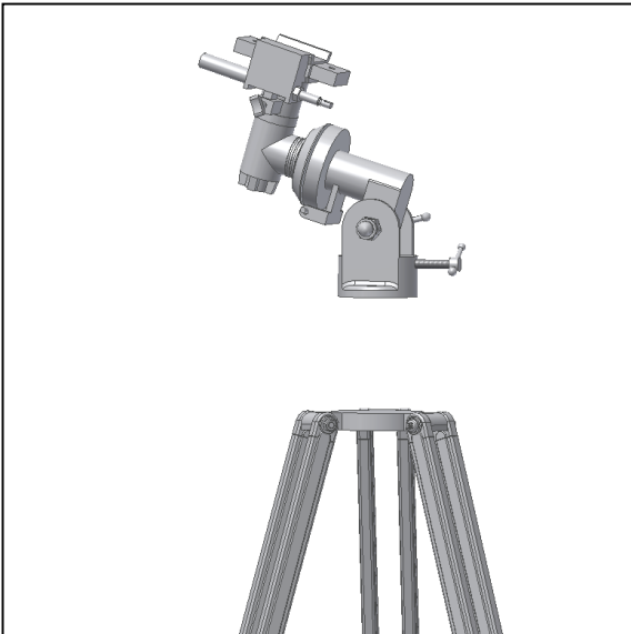
Figure 4. Place equatorial head on top of tripod.
